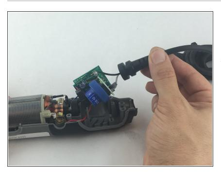
Using your fingers, carefully pull the circuit board from the casing. This will make it easier to remove the power cord.
