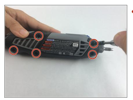
Using the Torx 15 screwdriver tip, remove the 5 screws (12.5 mm) that hold the casing together.
