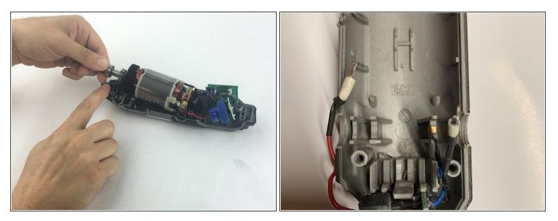
Carefully pull up on the shaft to lift out of the casing.
