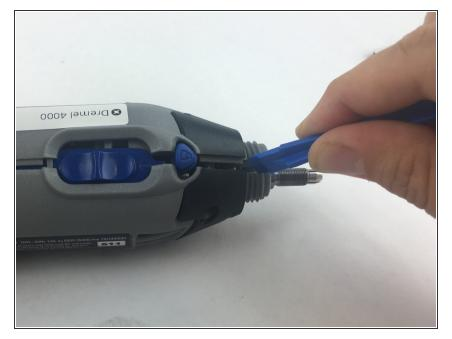
Use a plastic opening tool to gently wedge apart the hard plastic threads.
