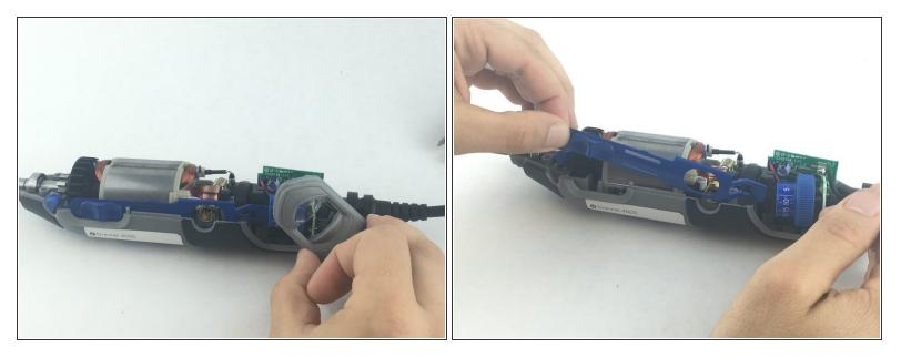
To clear access to the electrical assembly, remove the variable speed dial cap and blue power lever, and set them aside.
