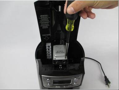
• Using the Crown Bolt #8 Steel Spanner, unscrew the four 8-mm screws labeled in a red outline.
