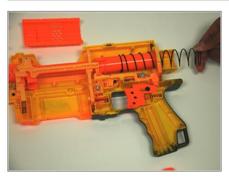
You should now be able to pull the primary firing spring from the rear of the rifle for replacement.
