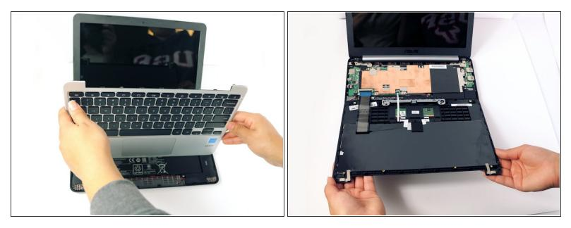
• Gently flip the keyboard cover away from the laptop. Rest it safely upside down so the cables are not strained and are easily accessible.
