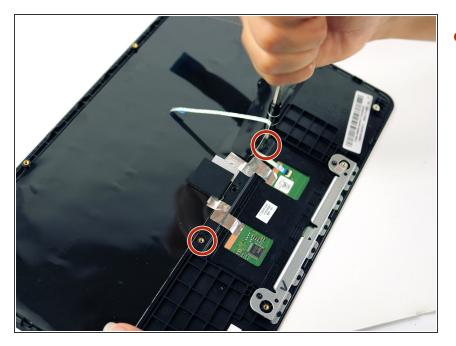
• Use a J0 screwdriver to remove the two 3mm JIS 0 keyboard screws.
