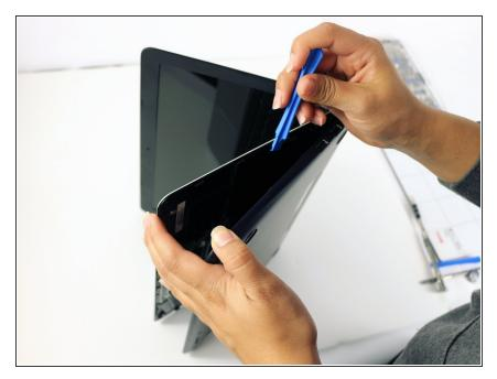
Turn the laptop on its side. Use a small, blue opening tool to pry the keyboard cover and laptop apart.
