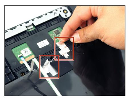
• Pull the tape connecting the keys from the palm rest assembly.
