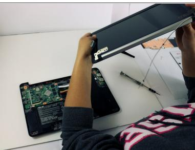
Carefully pop the LCD screen assembly out of the laptop case.
