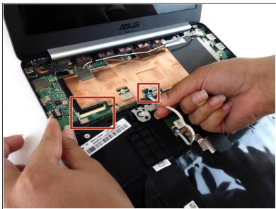
Carefully pull the keyboard cables out of the connecting ports that are attached to the motherboard.
