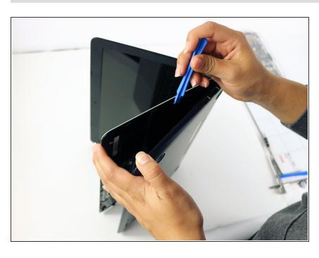
Turn the laptop on its side. Use a small, blue opening tool to pry the keyboard cover and laptop apart. Begin from the top right, next to the power button, and slowly work your way around to the opposite side until the keyboard cover is detached.
