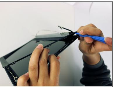
• Use a blue plastic spudger to snap the LCD cover off, working the spudger around the perimeter and completely remove the cover.
