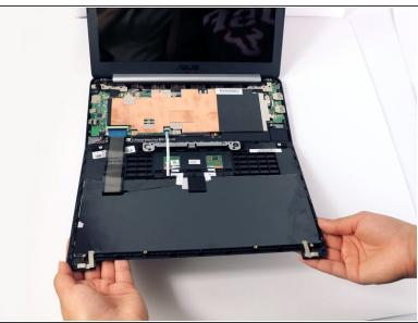
Gently flip the keyboard cover away from the laptop. Rest it safely upside down so the cables are not strained and are easily accessible.
