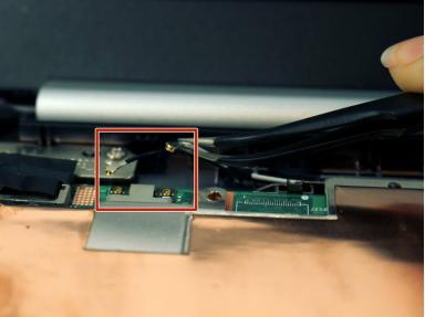
Disconnect the black and white cables located near the screen hinge.
