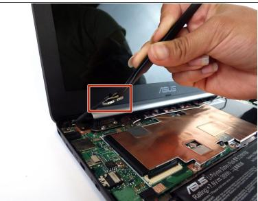
• Locate the LCD cable and its connector which is located in the upper left hand corner of the computer. Carefully flip up the tiny tab and safely remove the cable using precision tweezers.
