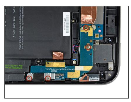
Remove the four 3.2 mm Phillips screws securing the USB connector board to the rear case.
