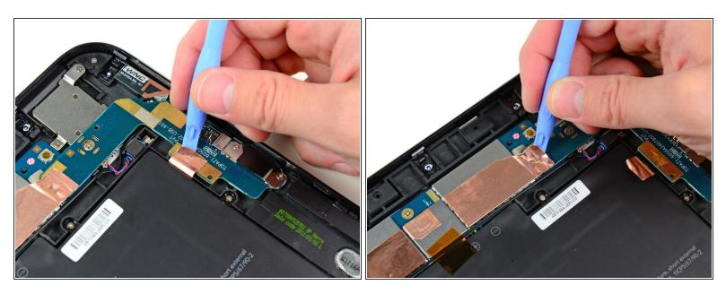
• Use the edge of a plastic opening tool to peel up the two pieces of copper tape covering the USB connector board near the battery and the motherboard.
