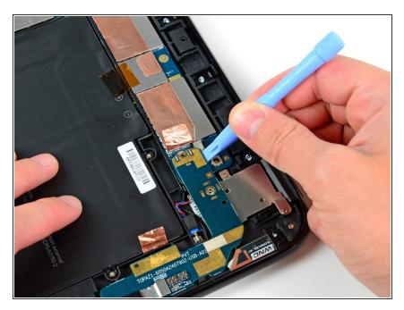
Pry the upper end of the USB connector board upwards to disconnect it from its socket on the logic board.
