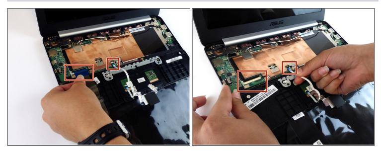
• Carefully pull the keyboard cables out of the connecting ports that are attached to the motherboard.
