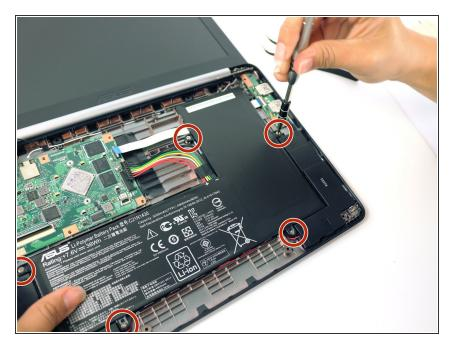
Use a J0 Phillips screwdriver to remove the 5, 4mm silver battery screws from the battery.
