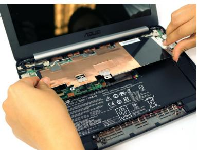
Use a J0 screwdriver to remove the seven 4mm silver heat shield screws and remove the heat shield.
