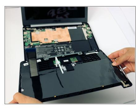
Remove the keyboard cover and safely place it somewhere face down.
