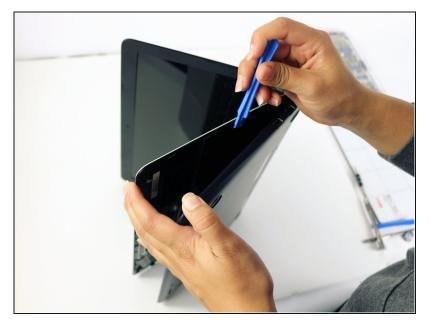
Turn the laptop on its side. Use a small, blue opening tool to pry the keyboard cover and laptop apart. Begin from the top right, next to the power button, and slowly work your way around to the opposite side until the keyboard cover is detached.
