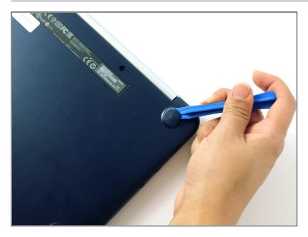
• Remove the two rear rubber feet by using one of the small, blue plastic spudgers.
