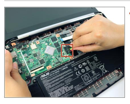
Pull the battery cable from the motherboard.
