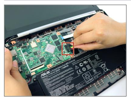
• Pull the battery cable from the motherboard.
