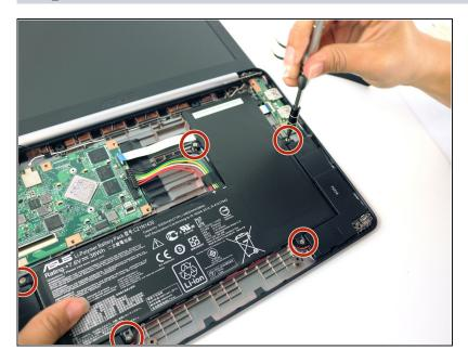
• Use a J0 Phillips screwdriver to remove the 5, 4mm silver battery screws from the battery.
