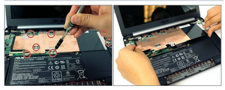
• Use a J0 screwdriver to remove the seven 4mm silver heat shield screws and remove the heat shield.
