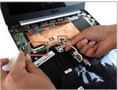
Carefully pull the keyboard cables out of the connecting ports that are attached to the motherboard.
