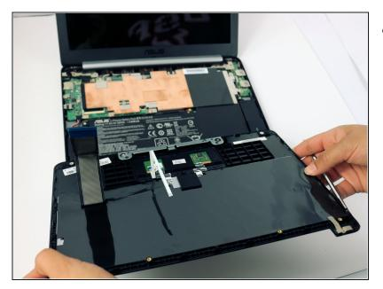
• Remove the keyboard cover and safely place it somewhere face down.
