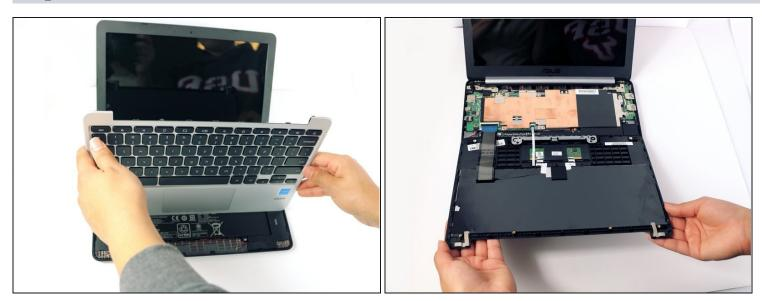
• Gently flip the keyboard cover away from the laptop. Rest it safely upside down so the cables are not strained and are easily accessible.
