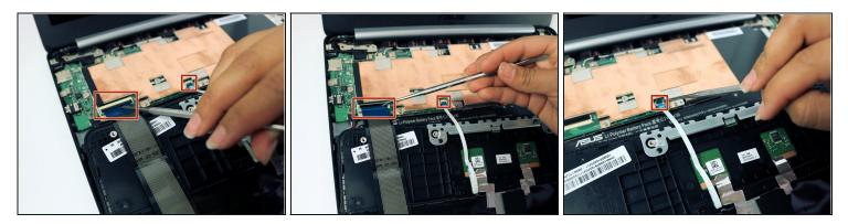
• Use the metal spudger to gently pry up the small tabs that are clamping down on the keyboard cables.
