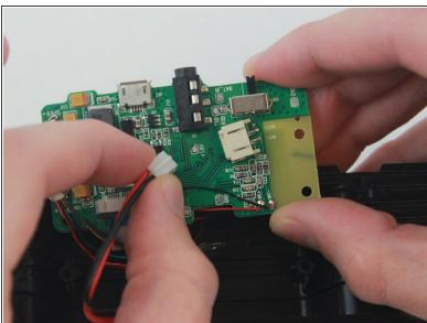
Disconnect the battery wires from the circuit board.
