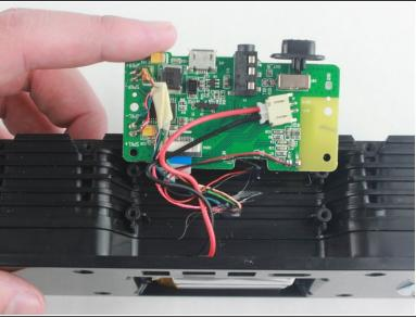
With the bottom plate removed now use the blue plastic opening tool to lift up the circuit board from the device.
