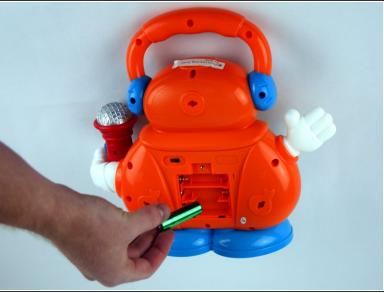
Remove the battery door and take out the batteries.
