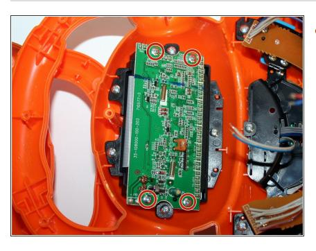
Using Phillips #1 screwdriver, remove the four 7.9 mm LCD board screws.
