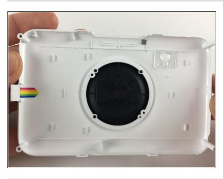
Remove the flash cover and place in the new one, with the holes of the flash cover oriented in the top right and bottom left corners.
