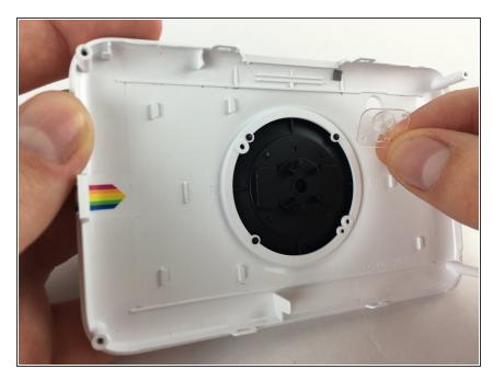
After the metal plate is removed from the front face-plate, locate the small clear flash cover on the top right of the faceplate. The flash cover should easily pop out of place.
