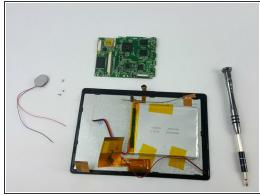
Use Phillips #J0 Screwdriver to remove three 1mm screws from the motherboard
