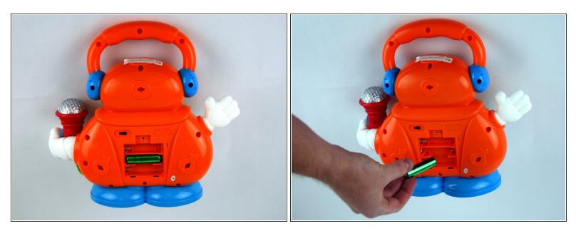
• Remove the battery door and take out the batteries.
