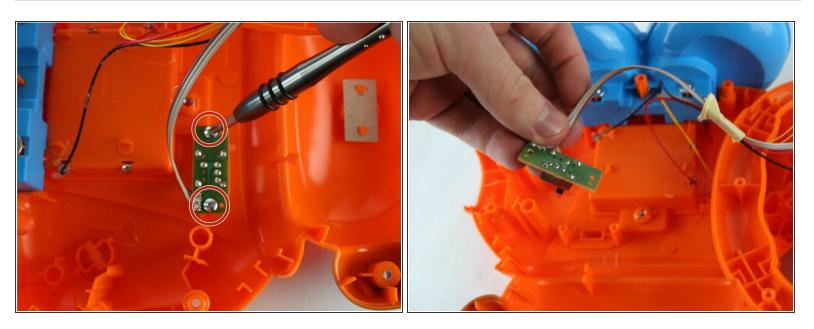
Using a Phillips PH1 screwdriver, remove the two 7.9 mm volume switch board screws.
