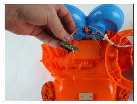
Once the screws have been removed, carefully move the volume switch board.
