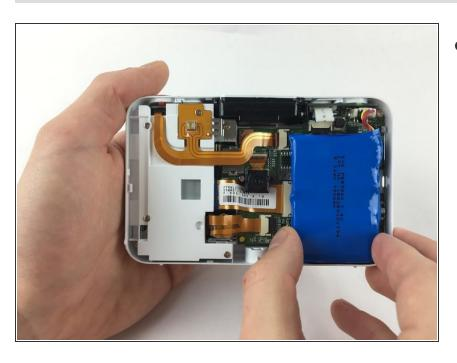
Two foam strips and adhesive glue binds the battery to the camera.
