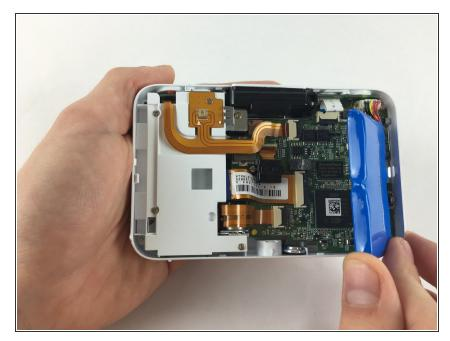
Remove the battery by lifting up the battery from the left corner. If you can not remove the battery with your hands, consider using a Plastic Opening Tool
