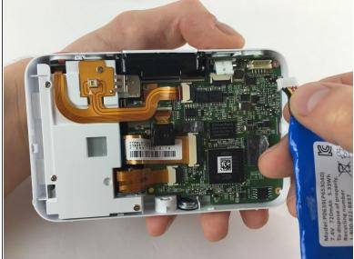
Using your fingers, remove the five pin connector from the device.
