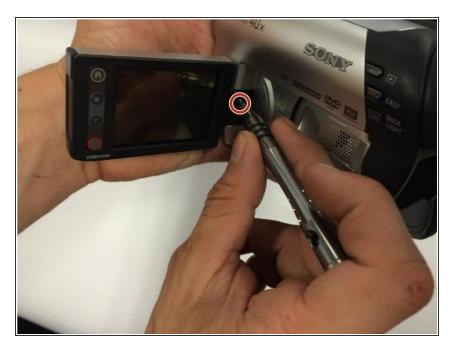
Remove the front facing screw adjacent to the LCD screen using a J1 Phillips screwdriver. The screw is 2.8 mm in length.
