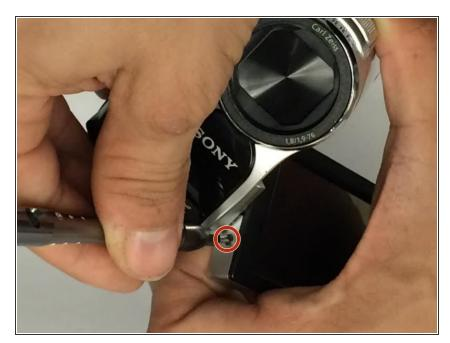
Rotate the camera screen until the screw on the bottom is clearly visible, then unscrew with a Phillips #1 screwdriver. This screw is 2.8mm in length.
