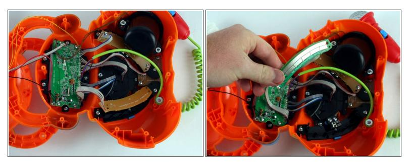
Once the screws have been removed, carefully move the mode switch board to expose the mode switch assembly underneath.
