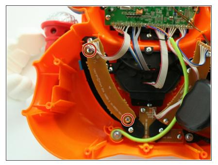
• Remove the two 7.9 mm Phillips #1 mode switch board screws.
