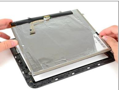
Lift up the LCD assembly and remove it from the front panel.
