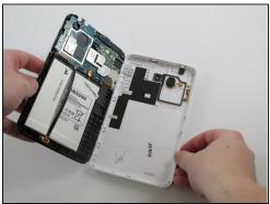
• After separating the tape holding the screen and case together, slowly start taking the screen off the case from the opposite side of the side with the buttons
