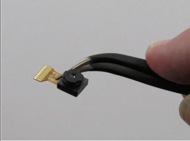
Using precision tweezers, gently pull the camera off the motherboard.
