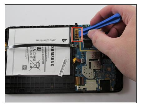
Use the plastic opening tool and gently pry up the tab holding the motherboard in place.
