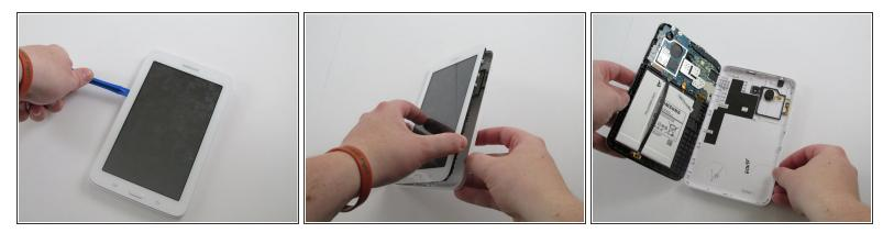
• After separating the tape holding the screen and case together, slowly start taking the screen off the case from the opposite side of the side with the buttons
