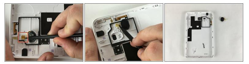
Using a spudger, carefully pry up the speaker ribbon cable.
