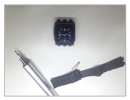
The first step is to remove the strap.
