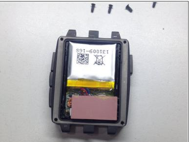
We will place this rubber in the lower right corner of the watch, on the vibrator and the connector of the screen. The golden connector on the left must be left free since it makes contact with the lid.
