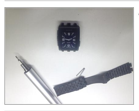
Finally we assemble the clock reversing the steps. '++ It is important when placing the cover to put first the two screws above and then the two screws below.' (This forces the entire internal chassis, thus exerting a pressure on the rubber contact of the screen.)
