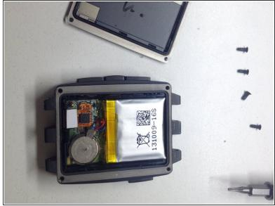
We will disassemble the cover of the clock using a screwdriver T-5, and being careful with the rubber gasket that has, we will remove the metallic cover.
