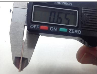
In this step we will look for a dissipative silicone of those that carry the laptops for the microprocessor. If you do not have it, you could use a piece of soft rubber that does not exceed 0.65mm thick.
