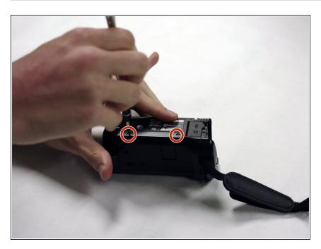
With the bottom of the camera facing up, remove the two 5.5mm Phillips #00 screws.
