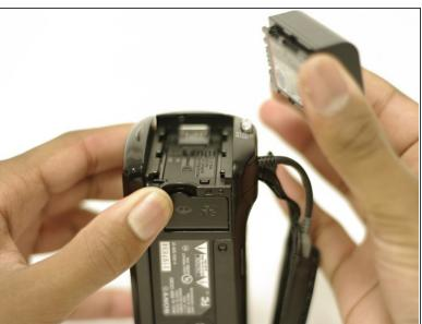
Using your right index finger and thumb, pull the battery toward you and then away from the camera.
