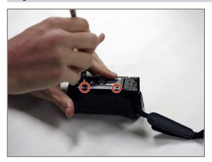
With the bottom of the camera facing up, remove the two
