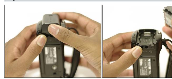
• Using your right index finger and thumb, pull the battery toward you and then away from the camera.
