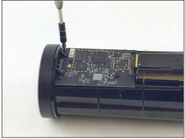
• Remove the four 9.7 mm T10 screws.
