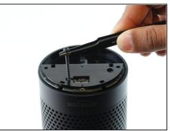
• Remove the four 42.8 mm T10 Torx screws from the bottom of the Echo.
