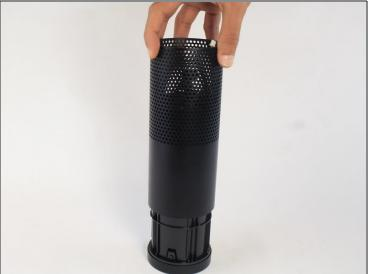
• Remove the plastic plate from the bottom of the device. Then remove the plastic shrouding.
