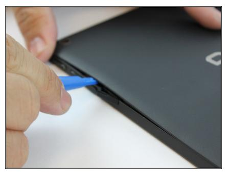
Starting at the Micro SD Card Slot and using the blue plastic opening tool, begin to maneuver the tool around the edges while applying light pressure to lift the panel upwards.
