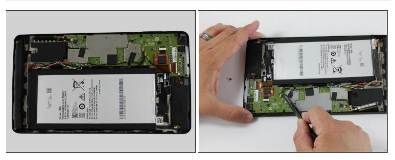
• Using the tweezers or your fingers lift the remaining black wires from the motherboard.
