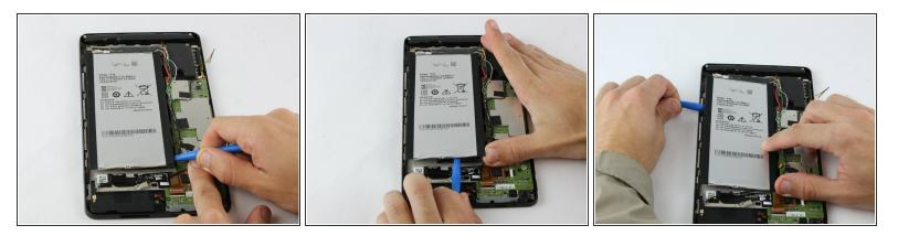
• Once you have the blue plastic opening tool underneath the battery, work the tool around the edges of the battery similar to the technique used for the back panel.
