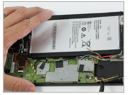
Using the angled tweezers, begin removing the antenna from the device.
