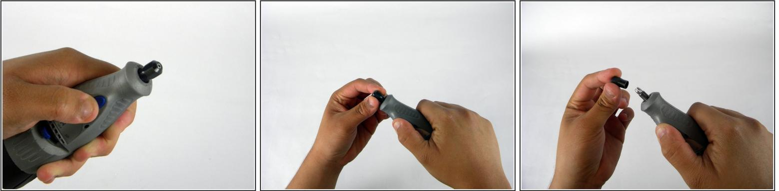
**i** The device comes with a small black wrench to tighten the collet nut, during reassembly or changing the bits.
