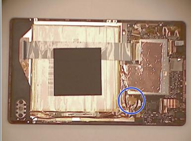
The connector slides out towards the outside of the device, and mine was pretty sticky so be careful.
