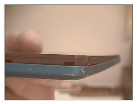
Wedge between the frame and back cover with an isesamo and separate all of the retaining clips
