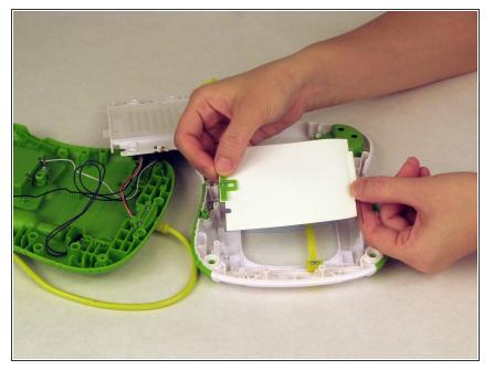
• Carefully remove the display screen, leaving the eraser slider attached.
