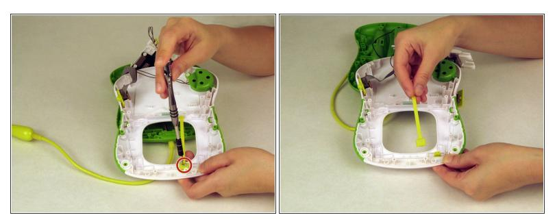
Use the Phillips #0 screwdriver to remove the eraser slider.
