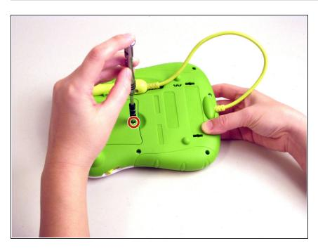
Use a Phillips head screwdriver to remove the screw from the battery compartment on the back of the toy.
