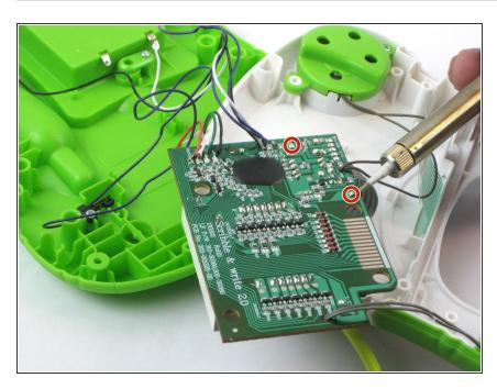
Remove the speaker wires from the motherboard with your soldering iron.
