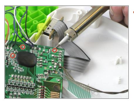
Remove the battery wires from the motherboard with the soldering iron.
