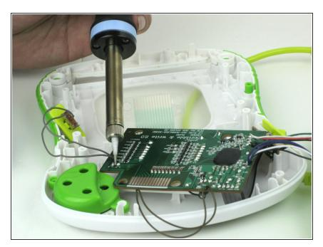
Remove the switch wires from the motherboard with the soldering iron.
