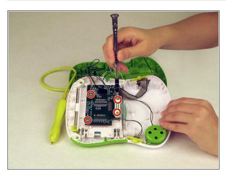
Using a Phillips screwdriver, remove the four screws from the motherboard.
