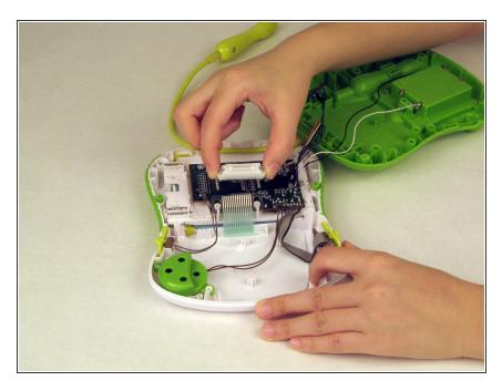
Remove the keyboard ribbon from the motherboard.
