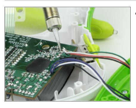
Remove the pen wires from the motherboard with the soldering iron.
