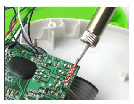
Remove the volume control switch from the motherboard with the soldering iron.
