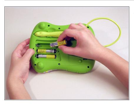
Remove the back battery cover and all of the batteries.
