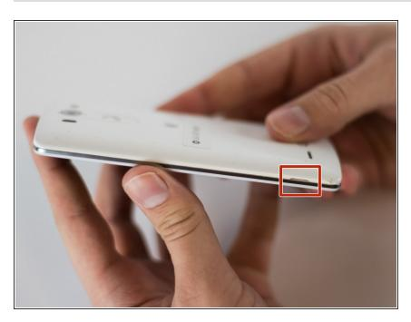
Locate the notch on the bottom right of the phone.
