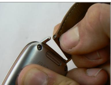
On the strap there is a knob. Sliding this knob towards the opposite side of the strap releases the tension on the spring bar, allowing you to pull the strap out..
