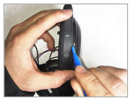
Use the plastic prying tool to gently remove the face of the speaker from the body.
