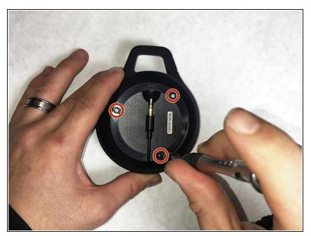
There will be three 6mm philips head screws under that rubber bumper, remove these three screws.
