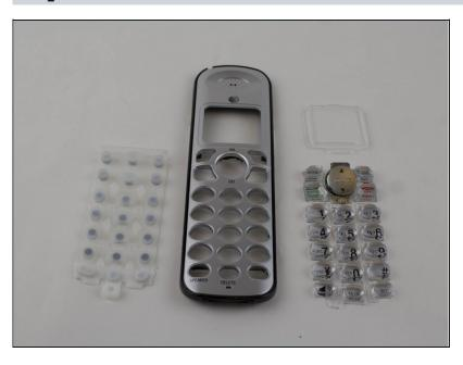
Replace the plastic display screen, or the keypad buttons as needed.
