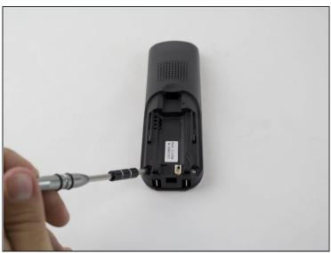
Remove the two 3.75 mm screws with a PH1 screwdriver.
