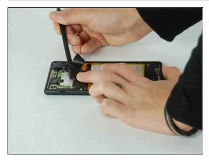
A Remove copper plated tape and any other securing adhesive with a nylon spudger. Remove carefully, as it has the potential or tear if too much force is used.
