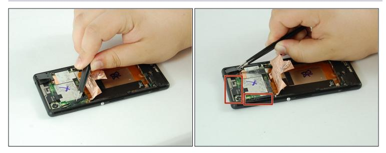
• Remove three pieces of the securing bracket using <u>tweezers</u>
