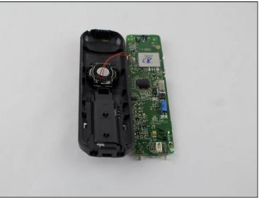
• Remove the two 3.65 mm screws on the motherboard with a PH1 screwdriver.
