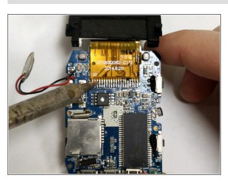
Using a soldering iron, melt the solder connection between the screen's ribbon cable and the motherboard. Pull the ribbon cable away before the solder solidifies. To reassemble your device, follow these instructions in reverse order.
