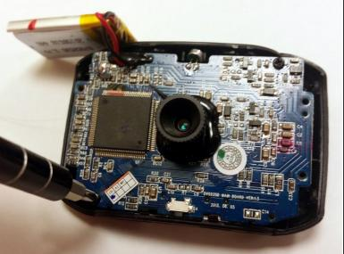
• Remove the two 4mm Phillips #1 screws holding the screen assembly to the motherboard.
