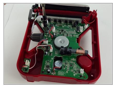
Remove the two 1 cm Phillips #0 screws that secure the tuning dial panel to the motherboard.
