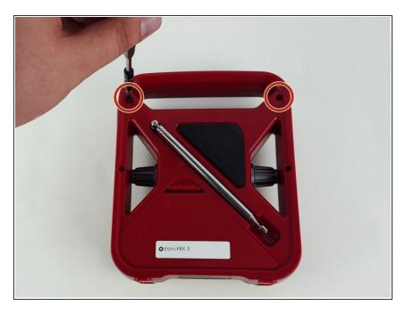
While using the T10 screwdriver, remove the two T10 screws on the back of the device's case.
