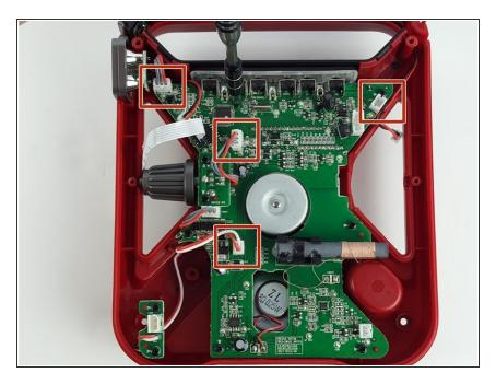
Unplug all the component socket connections from the motherboard.
