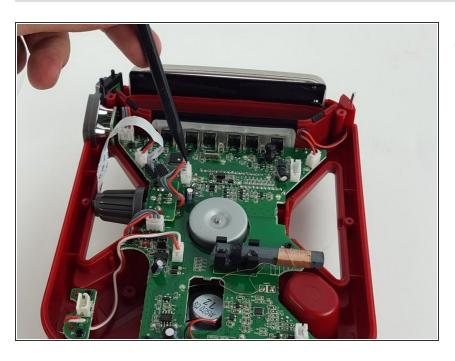
Unplug the socket connection from the motherboard as shown in the image.
