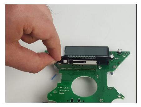
On the back of the motherboard, just below the LCD screen, gently pull up on the small, black plastic switch to remove it.
