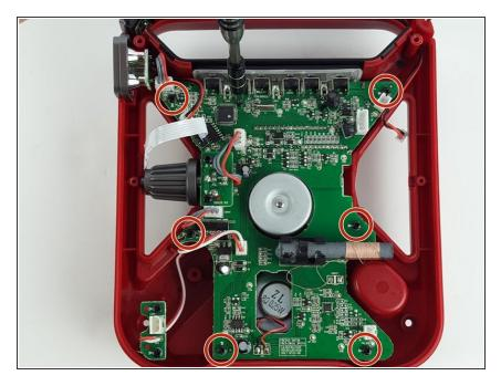
Remove the six Phillips #0, 1 cm screws that secure the motherboard to the case.
