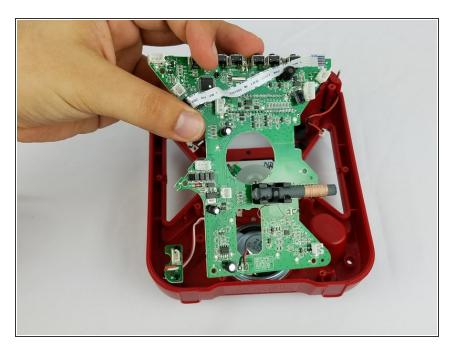
Gently lift the motherboard upwards to remove it from the device.
