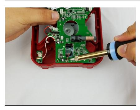
Desolder the two wires that connect the speaker to the motherboard.
