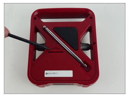
Pull the plastic tab on the battery compartment cover panel to loosen it, then pull the panel off.
