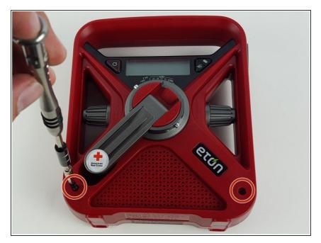
On the bottom of the device case's face are two T10 screws. Use a T10 Torx screwdriver to remove the two screws.
