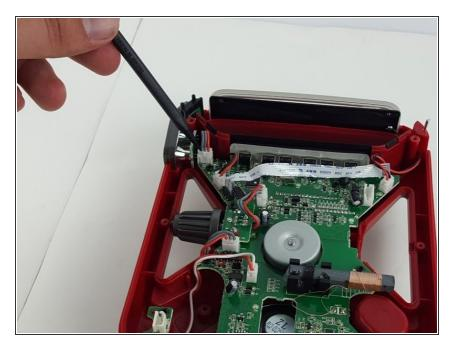
Pull the LED modules connector from its socket on the mother board.
