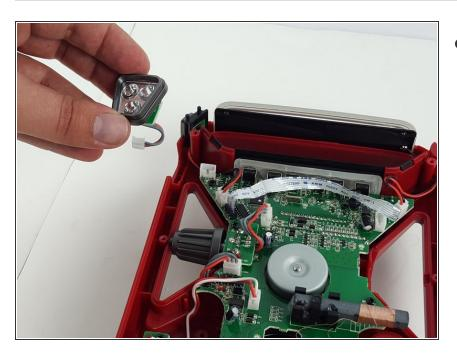
Gently lift the LED module upwards to remove it.
