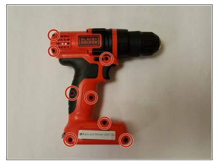
Rotate the drill to it's left side - the chuck should be facing rightward.
