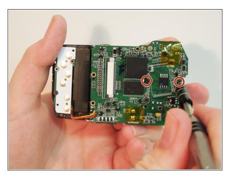
Remove the two screws holding the lens assembly to the motherboard using the PH00 bit screwdriver
