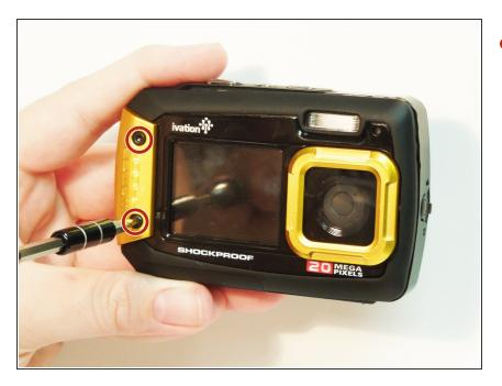
With the H2.0 bit screwdriver, remove the two screws on the yellow waterproof cover
