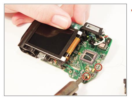
Remove the soldering on the 3 wires that are connected to the lens unit
