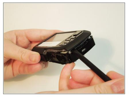
Pry off back outer casing using the black spudger or the blue prying tools
