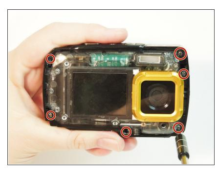
Remove the six screws from the edge of the clear inner casing with the PH00 screwdriver bit
