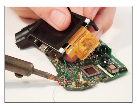
Remove soldering from the two green wires connected to the motherboard
