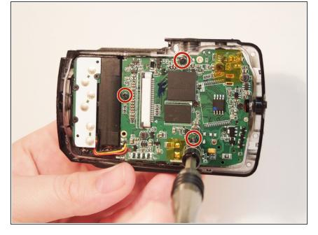
Remove three screws holding the motherboard into the casing using the PH00 bit screwdriver bit
