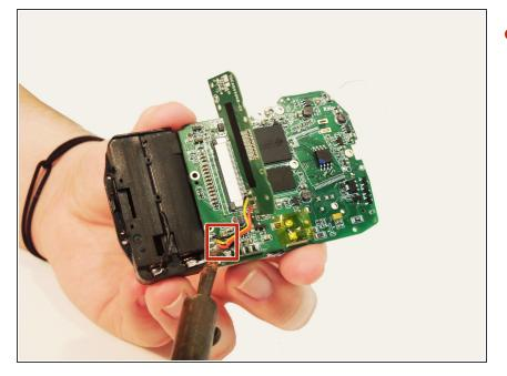
Remove soldering on the grouping of wires connecting the button sensors
