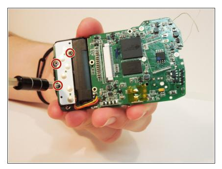
Remove the three screws holding the button sensors to the battery casing using the PH00 screwdriver bit
