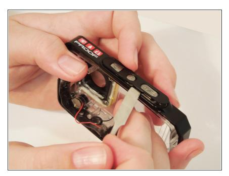
Use the metal prying tool to lift off the cover of the buttons
