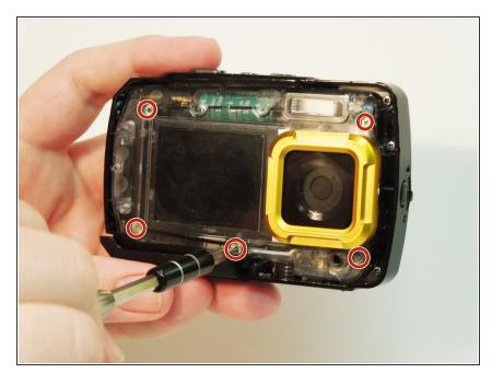
Remove the five silver screws from the inner casing using the PH00 screwdriver bit
