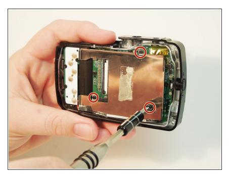
Remove three screws holding the silver screen casing to the motherboard using the PH00 bit screwdriver
