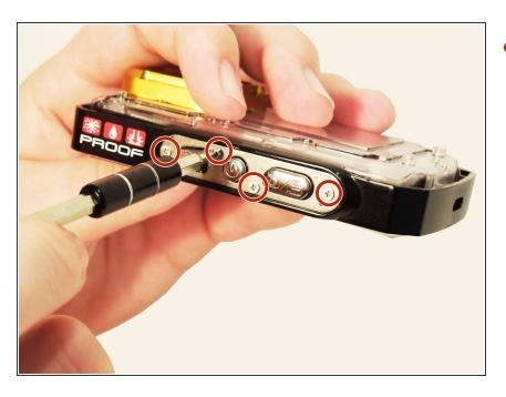
Use the PH00 bit to remove the four screws on the metal plate around the buttons
