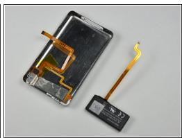
Be careful not to damage any of the headphone or battery ribbon cables while performing this step.
