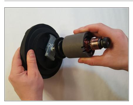
With a large amount of force, pull the motor up and off of the wire coil.
