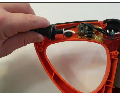
Gently pull the power cord out from the control module.
