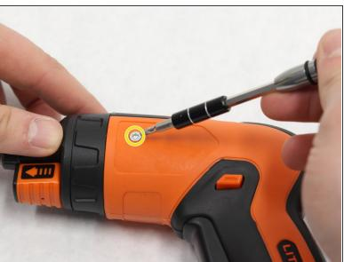
Remove the two screws that are 4-mm Hexagonal #2.5. These are very small case screws that can be found underneath the two stickers from Step 1.
