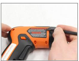
■ Remove the stickers found on the bottom and sides of the LI4000, using a spudger.
