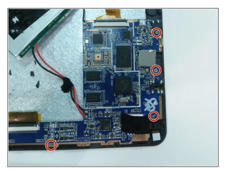
• Remove the four 2mm Phillips head screws from the motherboard.
