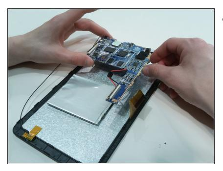
Remove the motherboard and battery from the back of the screen.
