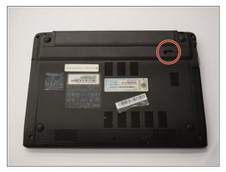
Locate the circular slot positioned at the bottom right of the battery.
