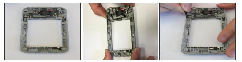
• Remove the volume buttons by pressing on the outer edge.
