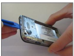
• Remove the six 1.4mm screws using a Phillips head screwdriver with a size PH00 bit. Then fully remove the back panel with a plastic opening tool.
