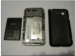
Use the curved opening at the center-bottom of the battery to carefully remove the old battery.
