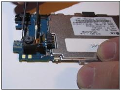
• The camera has been secured to the circuit board using an adhesive. Use a plastic opening tool and precision <u>tweezers</u> to remove it. Don't be afraid to use a little force when pulling at the camera.
