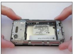
• Remove the six 1.4mm screws using a Phillips head screwdriver with a size PH00 head and remove the back panel with a plastic opening tool.
